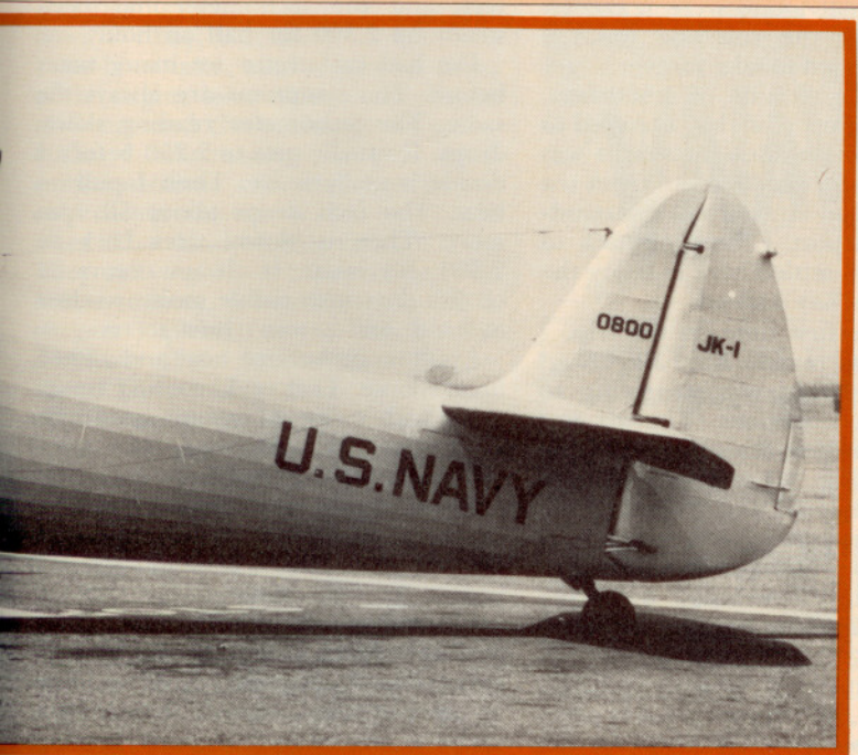
In postwar years, when 45A's were still useful workhorse airplanes and not yet treasured antiques, many individual modifications were made. This one has a metallized fuselage, modified windows, larger engine with constant-speed prop and modern avionics.
