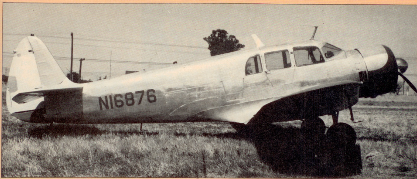
In postwar years, when 45A's were still useful workhorse airplanes and not yet treasured antiques, many individual modifications were made. This one has a metallized fuselage, modified windows, larger engine with constant-speed prop and modern avionics.
